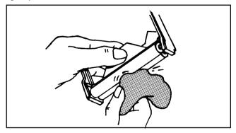
4 Replace the rollers by placing the assembly against the film exit door and rotating it downward.
